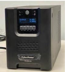
To set the unit for normal operation, press and hold the **POWER BUTTON** for five seconds. The unit will beep once. After approximately 10 seconds, the unit will briefly display **Operation Mode Inverter.** You should note that the "Output" voltage will now read **110Vac** instead of **000Vac.** The UPS is now in the operational mode with AC power provided to the Printer outlets, and battery backup is in effect if needed.
