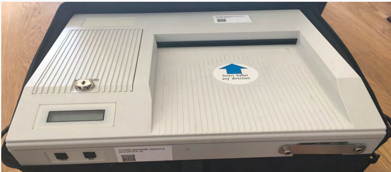
Picture: Originally marketed as Unisys ES-2000 later become Global Election Systems AccuVote-OS Precinct Count (AVOS-PC) paper ballot scanner. Later also marketed/supported under brands Diebold, Premier, ES&S and Dominion.
